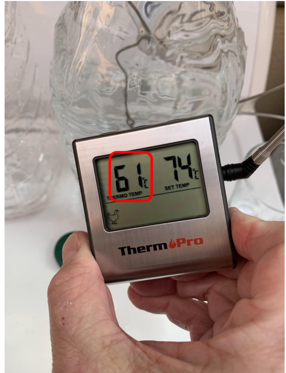
Hot Water Temperature: 61°C
